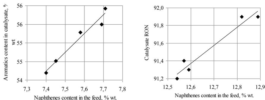
Fig. 3. Naphthenes content in the feed influence on aromatics concentration in catalysate and catalysate RON
