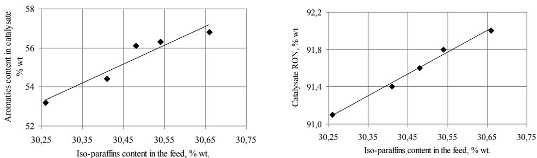
Fig. 2. Iso-paraffins content in the feed influence on aromatic content in the catalysate and the catalysate RON
