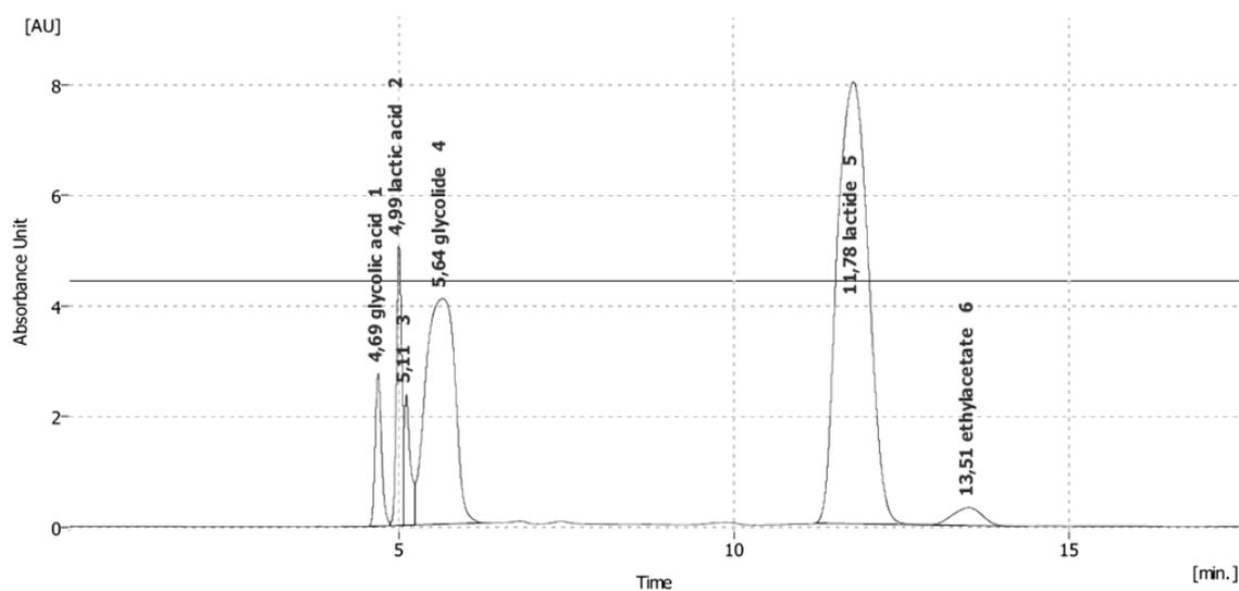
Figure 3. HPLC separation of glycolic acid, lactic acid, glycolide, lactide and ethyl acetate on Tracer Excel 120 ODSA, with  $c(\text{H}_3\text{PO}_4) = 3 \cdot 10^{-2}$  mol/L and column oven temperature  $40^\circ\text{C}$ , 200 nm.
