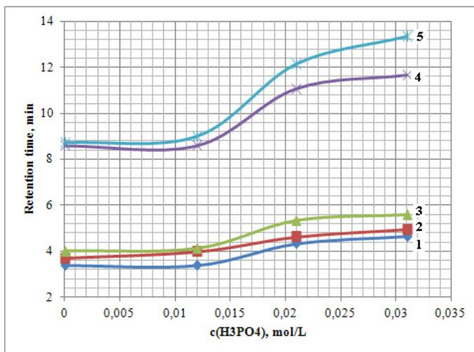
Figure 1. Influence of the  $\text{H}_3\text{PO}_4$  concentration of the mobile phase on the separation of GA (1), LA (2), glycolide (3), lactide (4) and ethyl acetate (5)
