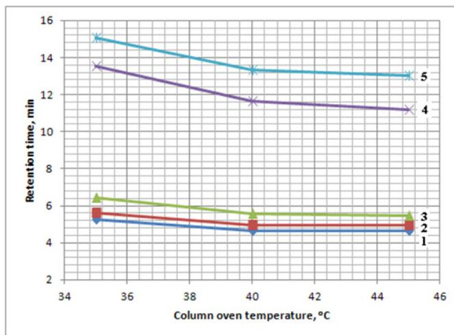
Figure 2. Influence of the column oven temperature on the separation of GA (1), LA (2), glycolide (3), lactide (4) and ethyl acetate (5)
