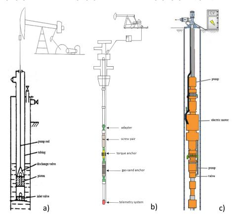
Fig. 1. Pumping units: a) piston sucker-rod pumping units (PSRPU); b) sucker-rod screw pumping units (SRSPU); c) electrical centrifugal pumping units (ECPU).
