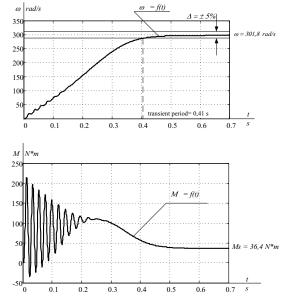
**Fig. 6.** The transient characteristics  $\omega = f(t)$ , M = f(t).
