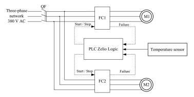
**Fig. 2.** Functional diagram of automatic cooling system: QF – the automatic circuit breaker, FC1 – the main frequency inverter, FC2 – the reserve frequency inverter, M1 – the main asynchronous motor, M2 – the reserve asynchronous motor PLC – the programmable logic controller Zelio Logic of Schneider Electric.
