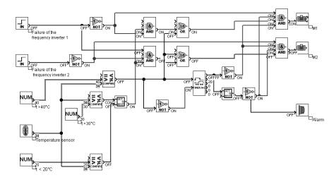
**Fig. 4.** The exterior of the software window of the PLC.
