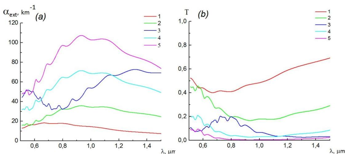
**Fig. The wavelength dependence of the extinction coefficient (a) and transmission function (b),  $h = 100 \text{ m}$ ; 1 –  $a=0.5 \text{ }\mu\text{m}$ ,  $C=5 \cdot 10^3 \text{ l}^{-1}$ ; 2 –  $a=0.7 \text{ }\mu\text{m}$ ,  $C=5 \cdot 10^3 \text{ l}^{-1}$ ; 3 –  $a=1 \text{ }\mu\text{m}$ ,  $C=5 \cdot 10^3 \text{ l}^{-1}$ ; 4 –  $a=0.7 \text{ }\mu\text{m}$ ,  $C=10^4 \text{ l}^{-1}$ ; 5 –  $a=0.7 \text{ }\mu\text{m}$ ,  $C=1.5 \cdot 10^4 \text{ l}^{-1}$ .**
