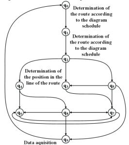
Figure 3. The scheme of the finite-state machine
