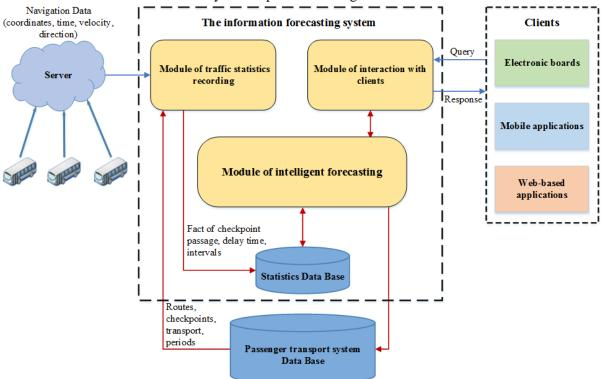
Figure 1. The structure of the forecasting system
