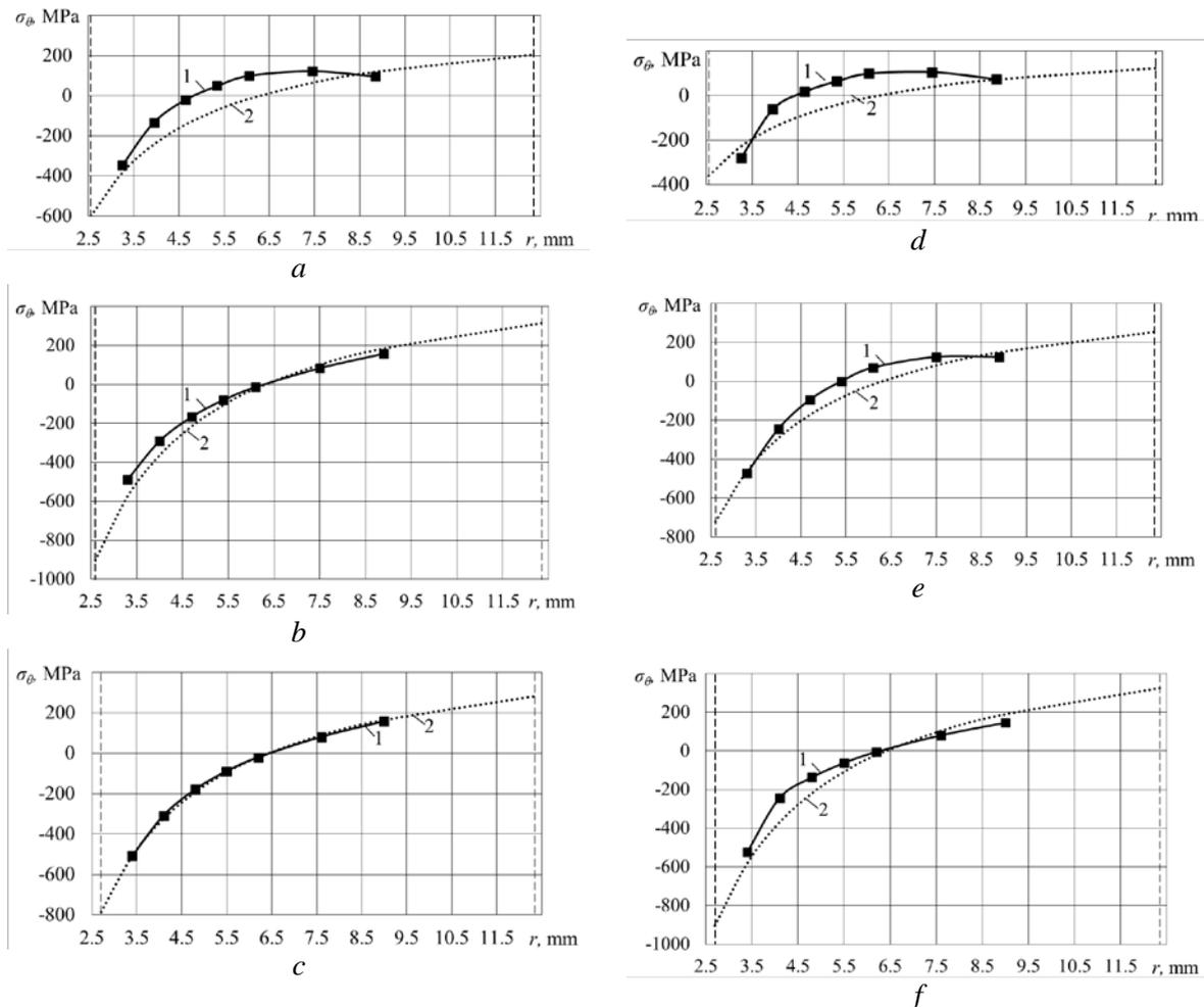
**Figure 6.** Curves for hoop residual stresses obtained by Sachs method (1) and by Davidenkov method (2), in the cold expanded samples with  $D = 25$  mm:
