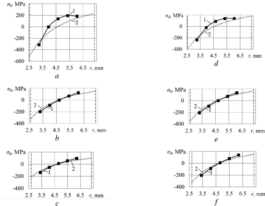
**Figure 5.** Curves for hoop residual stresses obtained by Sachs method (1) and by Davidenkov method (2), in the cold expanded samples with  $D = 15$  mm:
