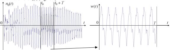
**Figure 2.** Function  $n_0(t)$  and wavelet w(t) formed on the basic function fragment.
