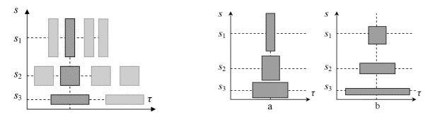
**Figure 3.** The window of wavelet timefrequency localization at different values of parameters of shift  $\tau$  and scale *s*. Figure 4. The window of time-frequency localization of wavelets with a number of periods equal to a) N=2 and b) N=8.
