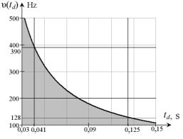
Figure 9. Dependence of boundary frequency of note pitch identification on its duration.
