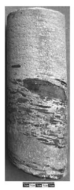
Obliquely laminated sandstone with level-by-level peb-Fig. 2. ble inclusions of clay rocks. The core, depth. 3113
