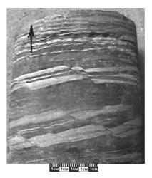
Fig. 3. Shift deformation of laminas in clay-siltstone interstratification. The core, depth 3066 m
