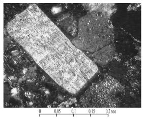
*Fig. 7.* Grains of feldspars changed in a different degree. The microsection, 2 nic., depth 3125.0 m
