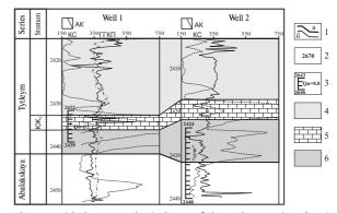
Fig. 1. Lithologo-geophysical cuts of the Tytleym series: 1) series borders (a), layers (b); 2) cable depth, m; 3) an interval of approbation and test results in the punched stem: Q<sub>μ</sub> – oil debit, m<sup>3</sup>/day; deposits: 4) clay-siliceous bituminous, 5) carbonate, 6) kaolinite-clay
