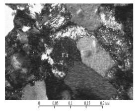
Fig. 8. Glauconite (GI). Contact cementation of fragments. The microsection, 2 nic., depth 3074,1 m
