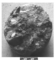
Basal conglomerate, main Core, depth 3141 m Fig. 1.
