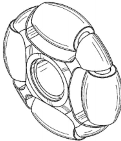
Figure 8. Omni-directional Wheel Rollers, the Axis of Rotation being located at an Angle of 90 Degrees to the Axis of Rotation of the whole Wheel
