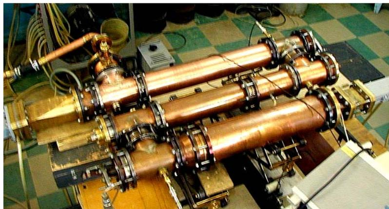
**Figure 4.** Active microwave compression system with a compact storage cavity in the form of a meander.
