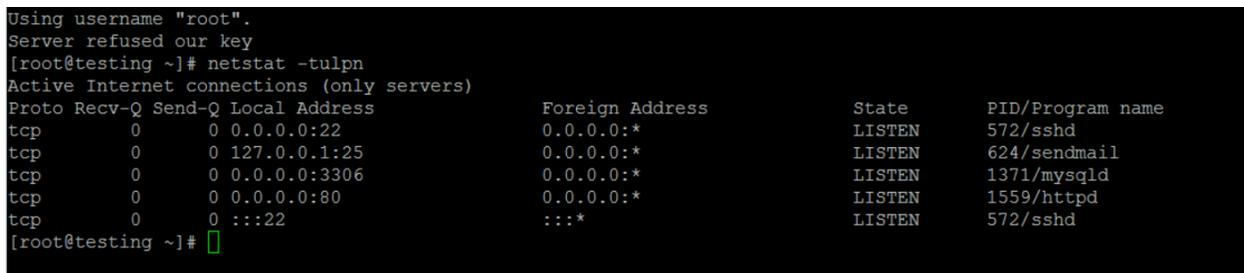
Figure 4.5 Verify installation of services
