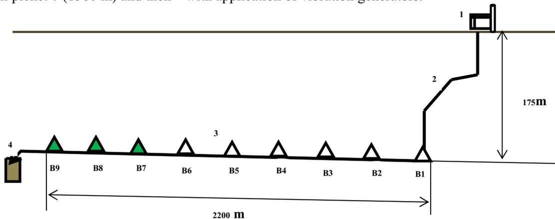
Fig.2. The diagram of vibration-pneumatic-gravity-flowing transportation of consolidating pulps from the stowing complex of Shokpak deposit to the shrink stoping of the deposit Kamyshovoye: 1 – stowing complex; 2 – vertical part of the pipeline; 3 – vibration generators; 4 – the stowing chamber of the block; B1-B9 – single-shaft vibration generators with electric motor drive
