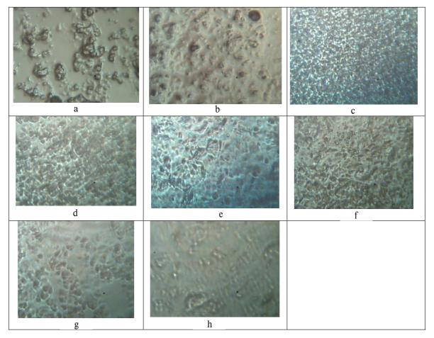
*Fig. 4.* Formation of paraffin hydrocarbon crystals in the deposit of the oil of 118 well (a−d) and 122 well (e−h) of Upper-Salat deposit at temperatures of oil stream and «cold rod»: a) 70 and 30 °C; b) 60 and 30 °C; c) 50 and 30 °C; d) 40 and 25 °C; e) 30 and 20 °C; f) 50 and 30 °C; g) 40 and 20 °C; h) 30 and 20 °C
