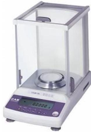
Figure 3.6 - Laboratory analytical balance CAS CAUW-120D
