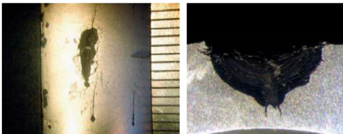
Figure 2.6 - Pitting and associated IGA/SCC in a VVER steam generator tube (IAEA, 2007).
