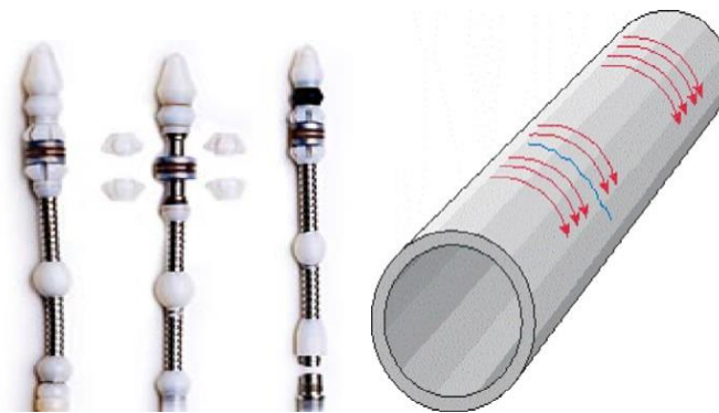
Figure 2.3 - Bobbin probes (A) view of typical bobbin probes for SG tubing inspection and (B) illustration of ET pattern generated by bobbin probes, demonstrating the limitations for detection of circumferential cracks.
