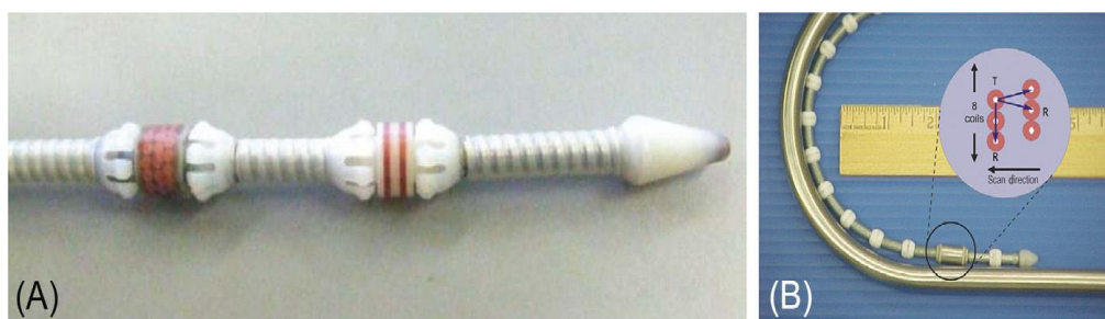
Figure 2.4 - X-probe for axial and circumferential crack detection (A) view of an X-Probe for 22.3 mm diameter tubing and (B) view of an X-Probe for 12.9 mm diameter tight-radius U-bend tubing.
