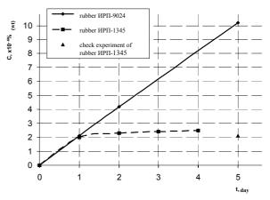
Fig. 2. Dependence of sulfur concentration in arsine on contact time with rubber samples
