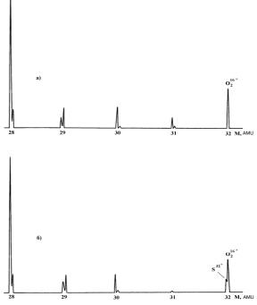
**Fig. 1.** Mass-spectra of purification plant fluxes: a) F, b)  $H_2$
