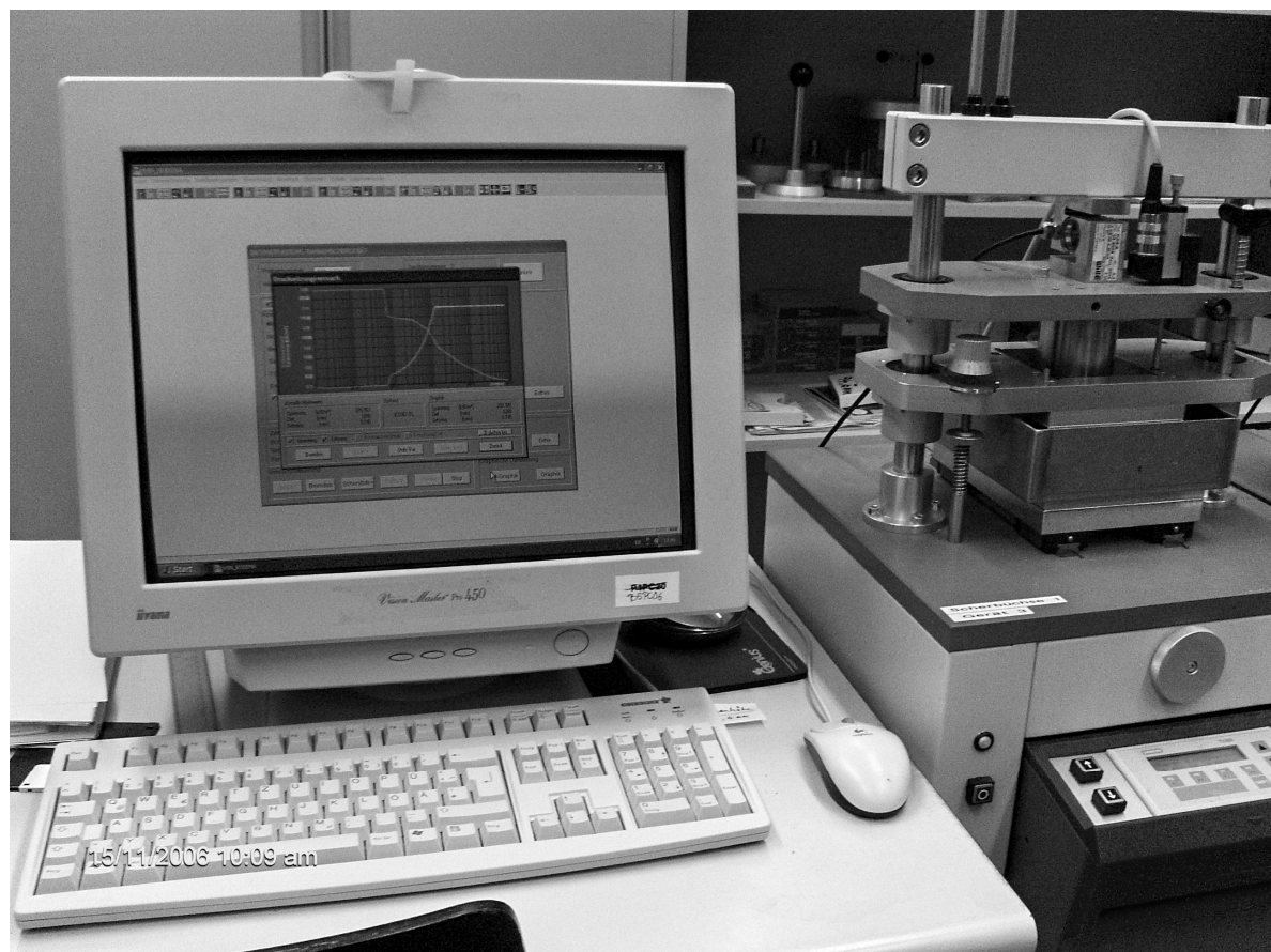
Fig. 1. The device for determination of compressibility and durability parameters made by Wille Geotechnik Company
