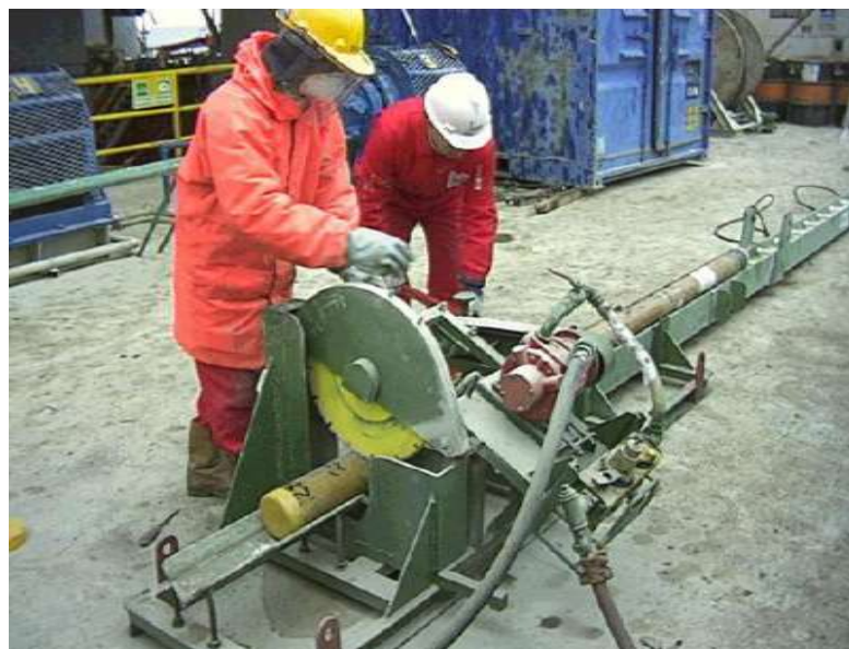
Fig. 2.6 - Segmentation of a core pipe
