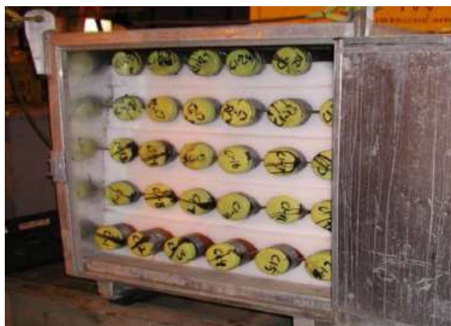
Fig. 2.9 - A special box for the transport of core tubes
