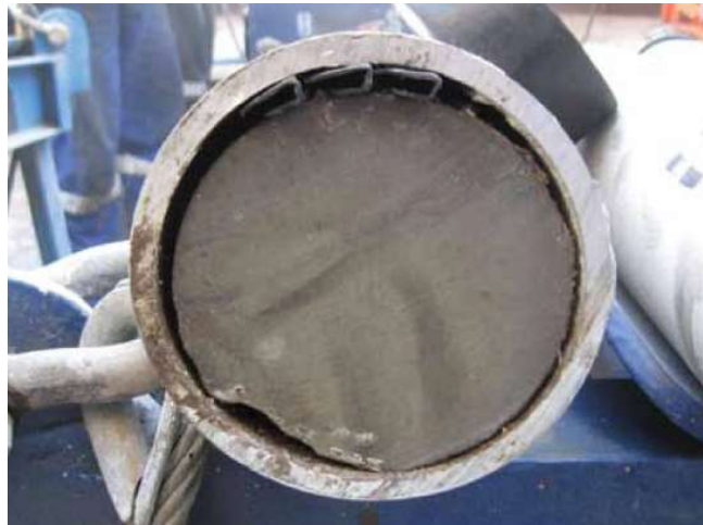
Fig. 2.8 - Core stabilization using Plastic Strip (Baker Hughes) technology
