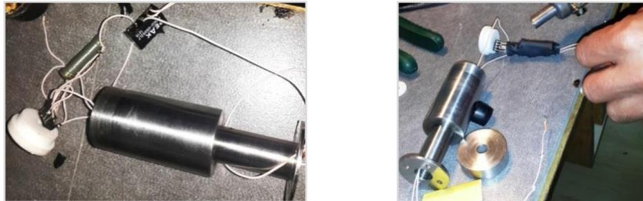
Figure 7 - Appearance of the pyrobolometer structure
