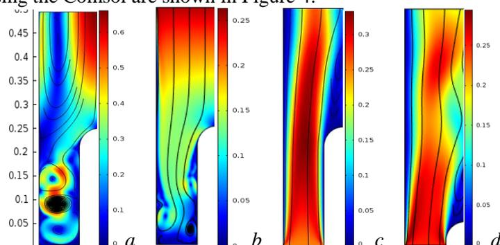
**Figure 4.** Gas flow diagrams in the chamber at the cylinder moving: *a, b* – up; *c, d* – down.
