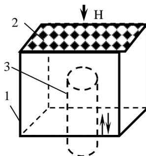
**Figure 3.** Measuring chamber scheme: 1 – chamber, 2 – perforation, 3 – mobile cylinder.
