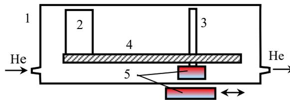
**Figure 1.** Experimental facility: 1 – chamber, 2 – sensor  $\alpha$ -particles, 3 – source  $\alpha$ -particles, 4 – rail, 5 – permanent magnet.
