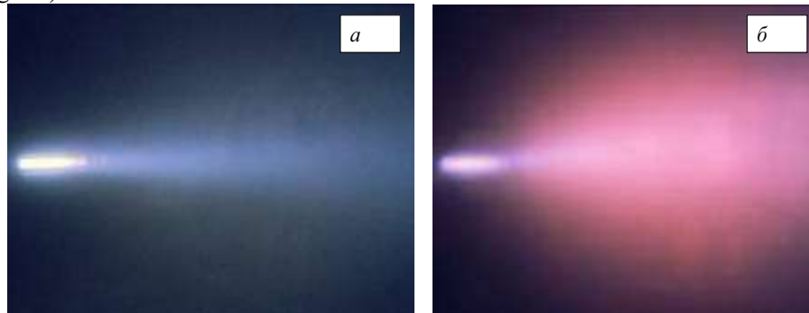
Fig. 2 Beam plasma glow at different beam currents: a - 200 mA, b - 250 mA.
