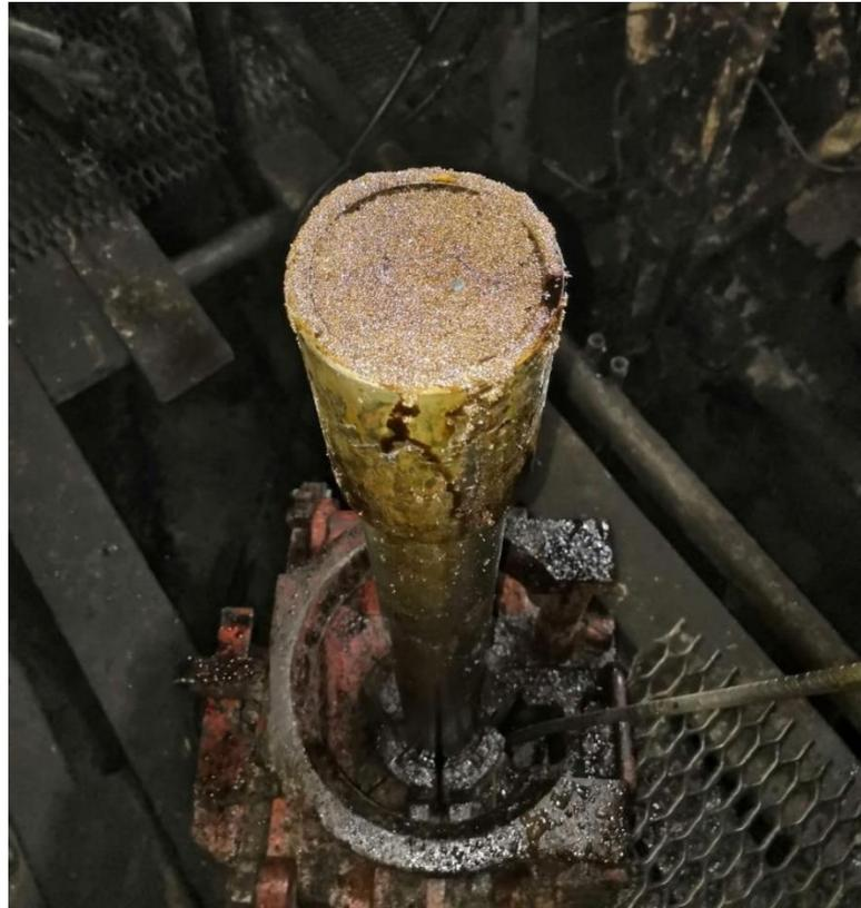
Figure 5 -Working stage of an electric centrifugal pump after clogging with proppant
