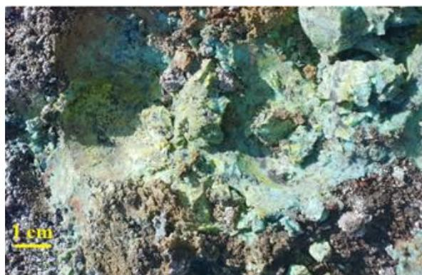
Fig. 1. Photograph of secondary sulfates on the heap surface
