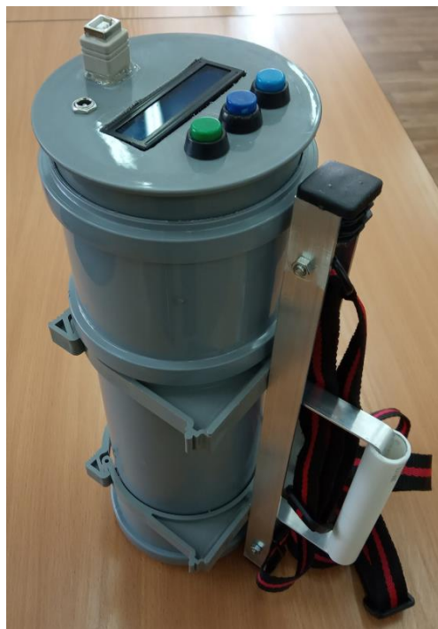
Figure 2.3 – Dosimeter based on a scintillation detector
