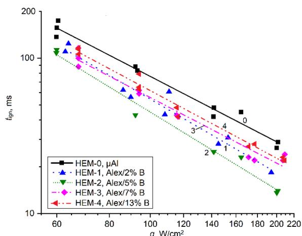
**Figure 1.** The ignition delay time of the HEM samples containing  $\mu\text{Al}$  and Al/B vs. the heat flux density.
