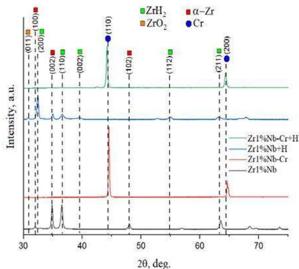
Figure 4. Diffraction patterns of the studied material of the Zr1%Nb-Cr with thickness of the chromium coating (9±1) microns
