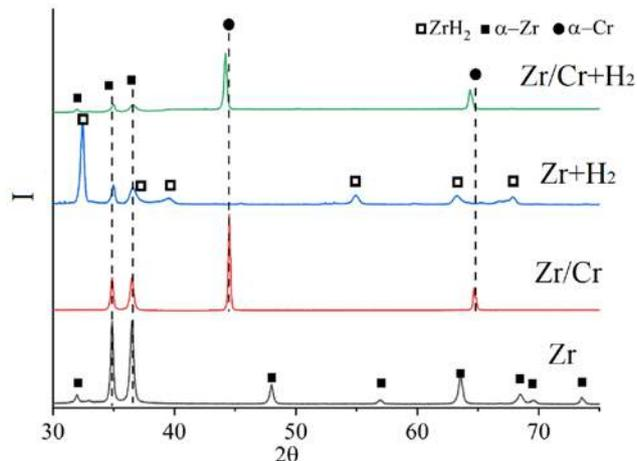
Figure 3. Diffraction patterns of the studied material of the Zr1%Nb-Cr with thickness of the chromium coating (6) microns
