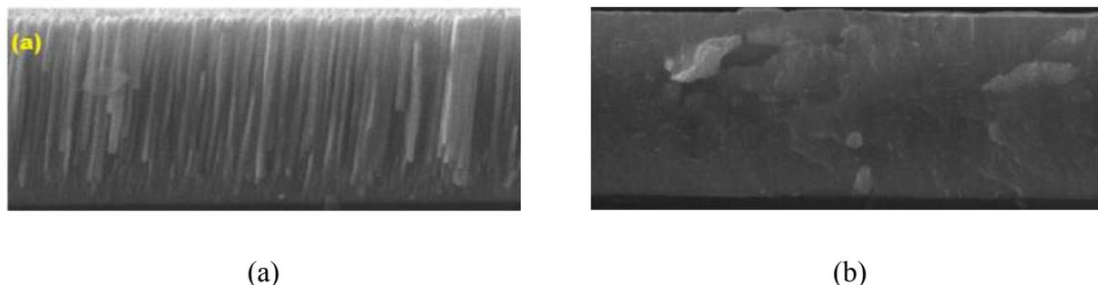
Figure 1. Image of metallographic sections of samples of Zr1%Nb zirconium alloy with chrome coatings obtained using MPC with “hot” (a); and in cooled targets(b)
