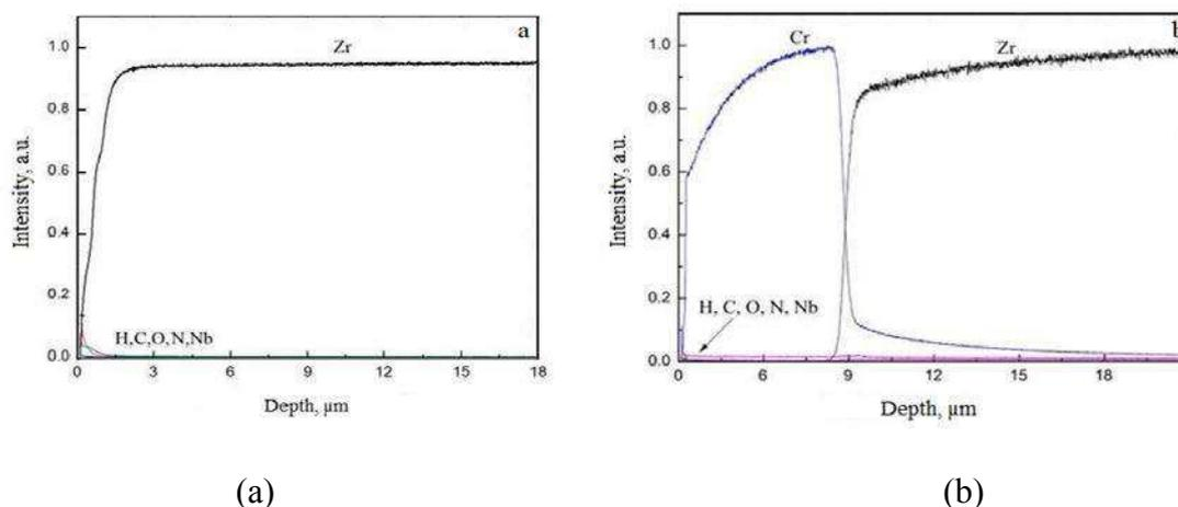
Figure 2. Depth distribution of chemical elements in the alloy Zr1%Nb (a) and Zr1%Nb-Cr (b)
