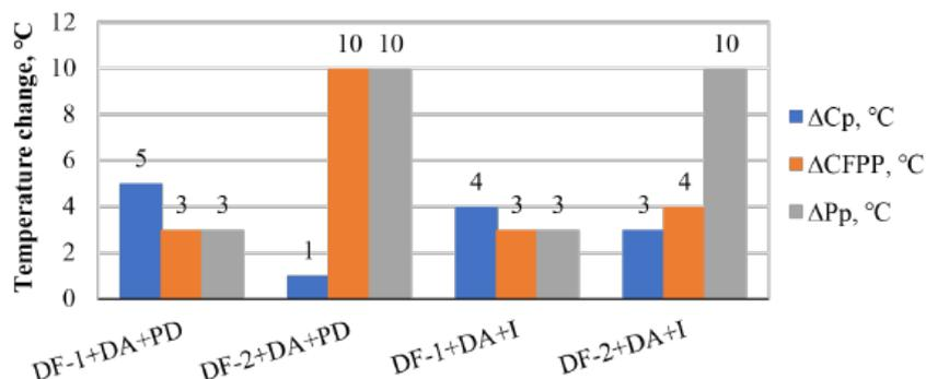
Fig. 2. Changes in the LTP of mixtures of DF with an additive when adding HTN
