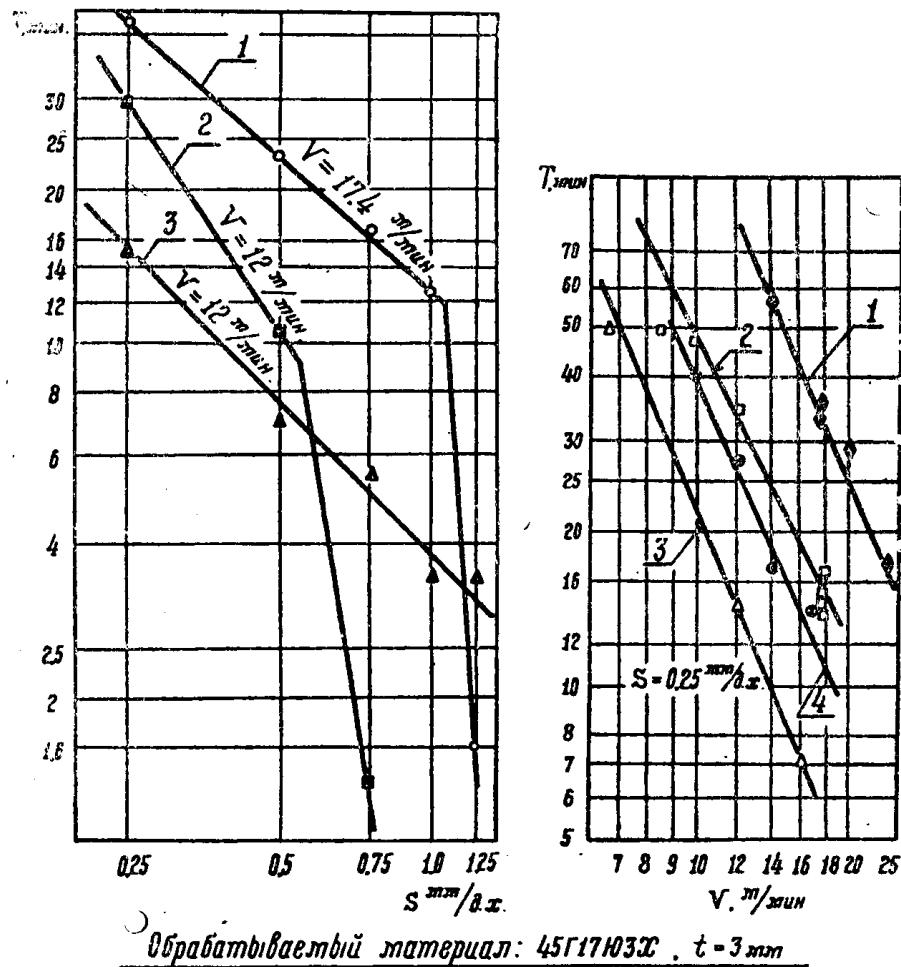
1.-Литой сплав Я:  $\alpha = 7^\circ$ ,  $\gamma = +14^\circ$ ,  $\lambda = +12^\circ$ ,  $\varphi = 40^\circ$
